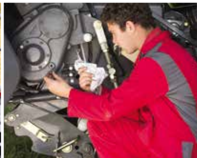
3. Checking the cutter gearbox oil level.
