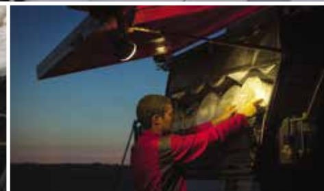
Twine box lighting allows easy night time refilling.
