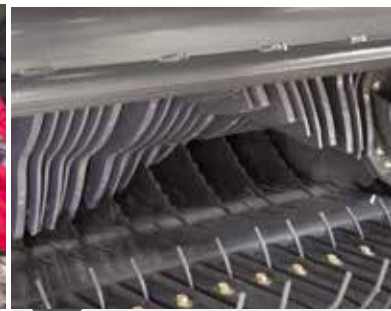
Heavy duty four-lobed spiral cutter rotor for smooth crop flow.
