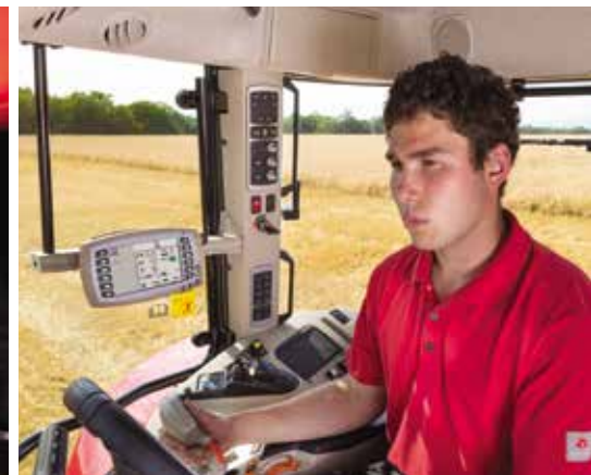
Controlling the baler via the tractor ISO VT terminal.
