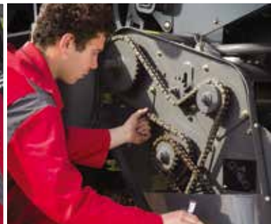
4. Checking the pick-up chain tensions.
