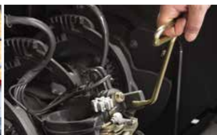
Each knotter head can easily be lifted for inspection and service.
