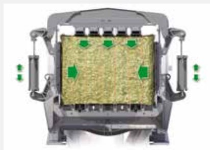
Three-way double acting density system.
