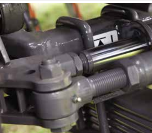
Rear axle hydraulic steering lock.
