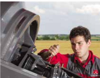
5. Adjusting the flywheel slip clutch.
